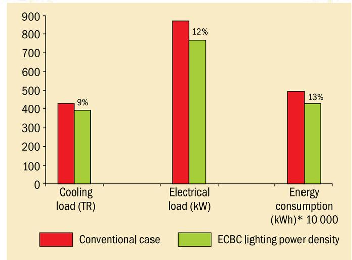
Figure 7 Impact of the ECBC lighting power density
