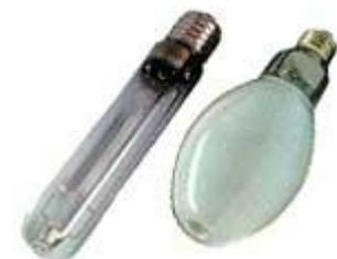
High Pressure Sodium vapor lamp is a gas discharge lamp which uses sodium in an excited state to produce light. The efficacy of HPSV varies from 50 -140 lumens/watt and lamp life is around 16000 - 24000 hrs. The color rendering index of these lamps is quite low. These lamps can be primarily used for applications where lighting from a height around 5m is desired such as for the drive ways in a campus or car parking etc.
